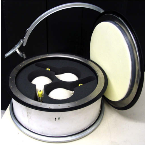
Fig. 1. Permanently magnetized spin box mark 3 for shipping hyperpolarized ^3\text{He} (Section 3.3). On the right leans the top cover which forms the second pole face, on the left the respective clamp ring. Inside one recognizes three flasks of 1.1 liter volume each, filled with hyperpolarized ^3\text{He} at a pressure of 2.7 bar and closed by a stop cock. A cover from flexible tissue protects the user from glass splinters in the case of bursting. The magnetic field is 0.8 mT. Within the volume occupied by the flasks, the relative field gradient is limited to \lesssim 10^{-3}/\text{cm} when the box is closed.
